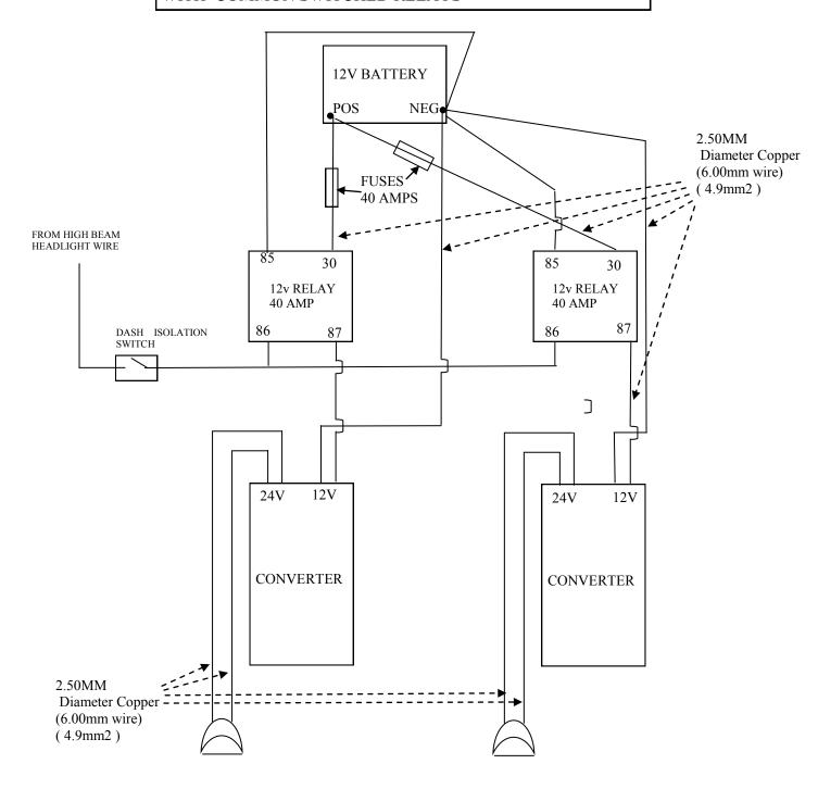
Note: 2.50mm Dia copper wire = approx (10 AWG = 6.00mm wire = 4.9mm2
